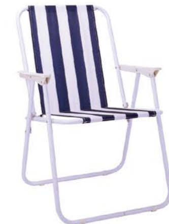
Fe YTBC055S Size: 53x46x76cm steel tube dia.18x0.8mm powder coated 180gsm polyester packing 58x35x69cm 10pcs
