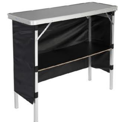
YTF106 Size: 99x38x52.5/90.5cm aluminum tube 25x25x1.0mm, oxidation 5 mm MDF with width 3.5cm aluminum surround 2pcs 210D walls; 600D polyester carry bag Packing 103x7x41cm 1pcs
