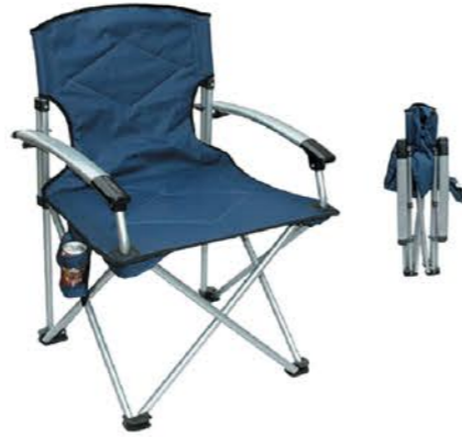
Fe ↔ ↔ YTBC077A Size: 65x64x48/95cm steel tube dia.19x0.9mm powder coated; Alu. armrest double 600D polyester with PVC coated; 1cm thickness sponge filling; with a side cupholder pocket Packing 90.5x33x41cm 4pcs
