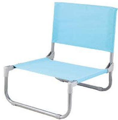
Fe YTBC067A Size: 50x45x50cm steel tube dia.18x1.0mm powder coated; solid color 600D Polyester with PE coated Packing 65x43x50cm 12pcs
