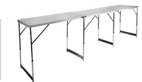
Ai ↔ YTFT020 Size: 240x60x55/62/70cm aluminum tube dia.25/23/19x0.8mm, oxidation 5mm MDF table top with 3.2cm aluminum surround Packing 62x14.5x63cm 1pcs
