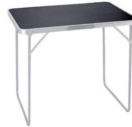
Ai ↔ YTFT016-70cm Size: 70x50x60cm steel tube for leg dia.16x0.6mm, powder coated; 5mm MDF table top with 3.2cm width aluminum surround Packing 71.5x27x52cm 6pcs
