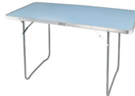
Ai ↔ YTFT016B Size: 120x60x70cm steel tube dia.16x0.6mm powder coated; 5mm MDF table top with 3.2cm width aluminum surround Packing 121x6.5x62cm 1pcs
